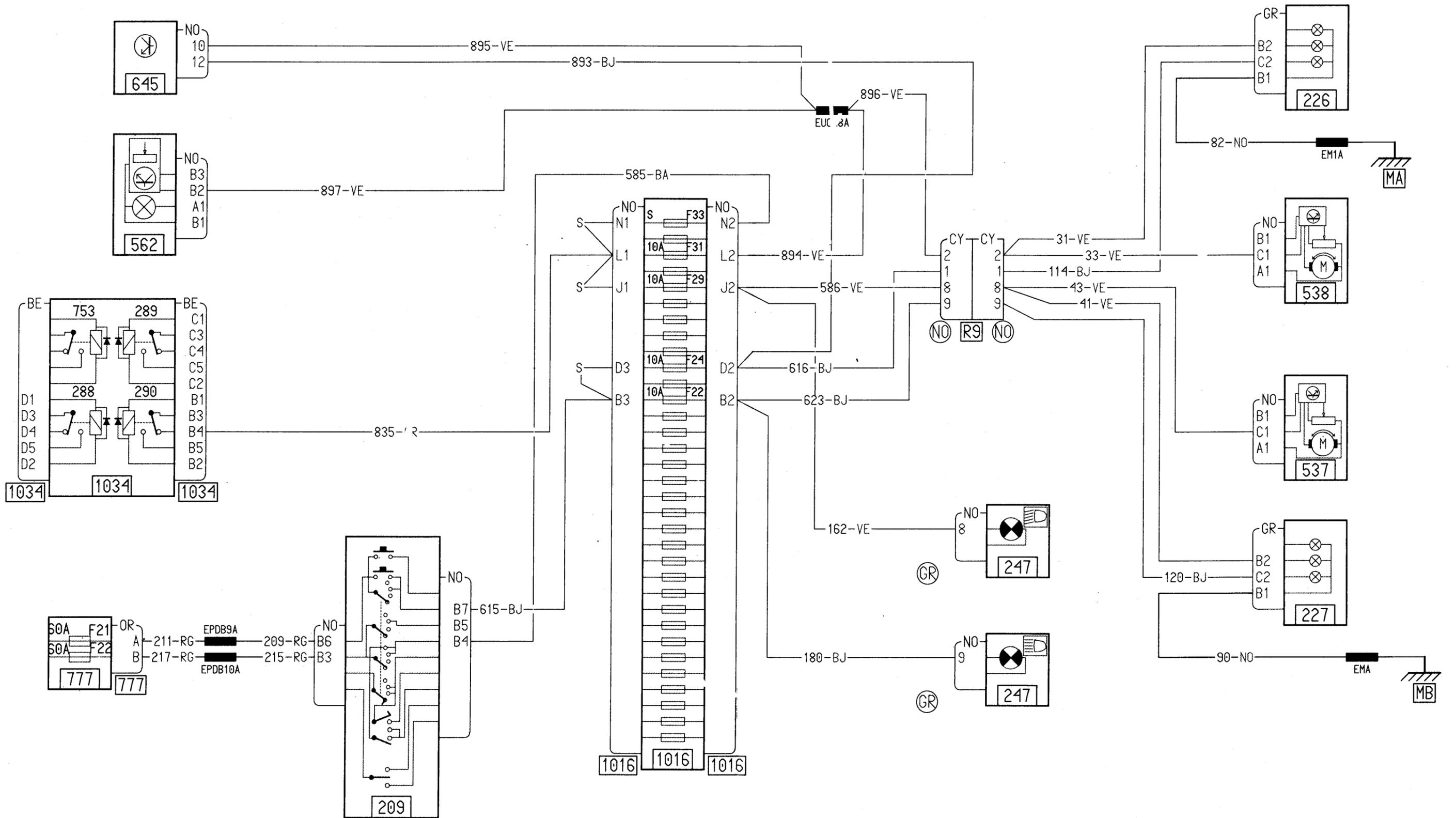
DIPPED BEAM HEADLIGHTS + MAIN BEAM HEADLIGHTS
