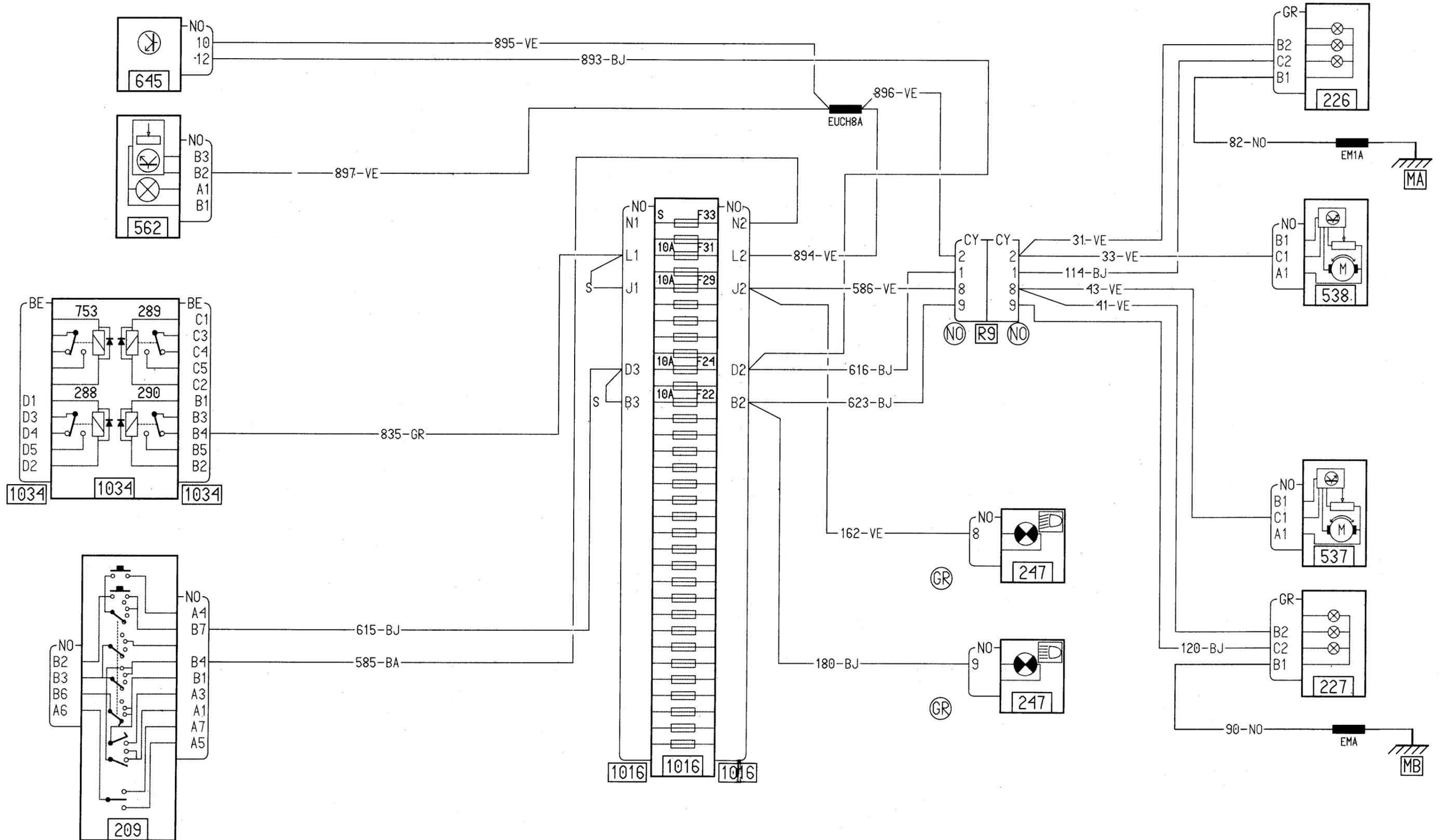
DIPPED BEAM HEADLIGHTS + MAIN BEAM HEADLIGHTS
