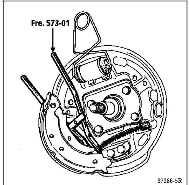
Remove all dust from the drums and backing plates using brake cleaner **Part Number 77 11 170 801**.
