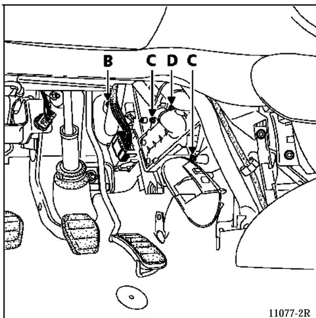
Separate the water downpipe from the matrix.
