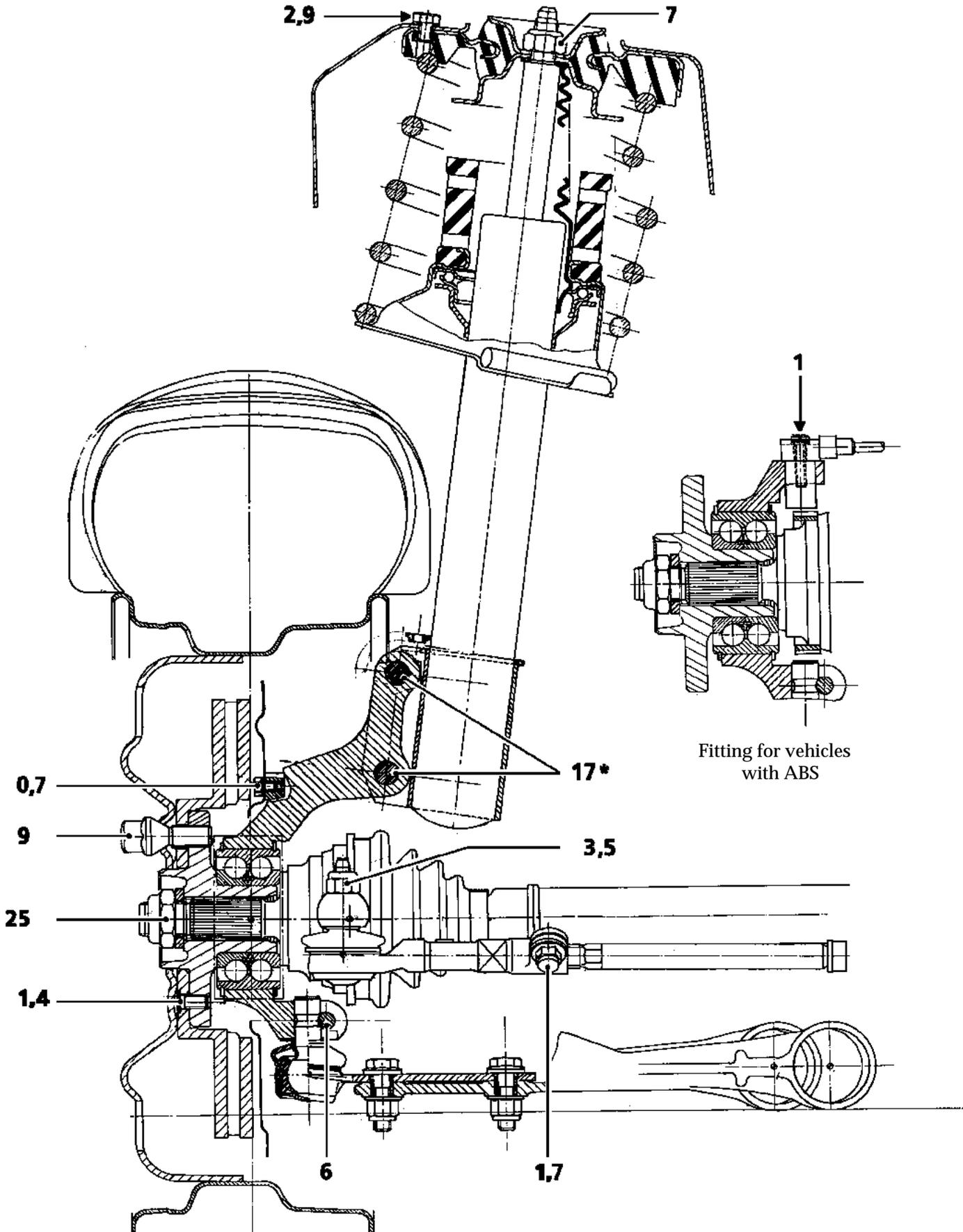
(\*) Fitting direction must be observed (bolt head next to brake caliper)
