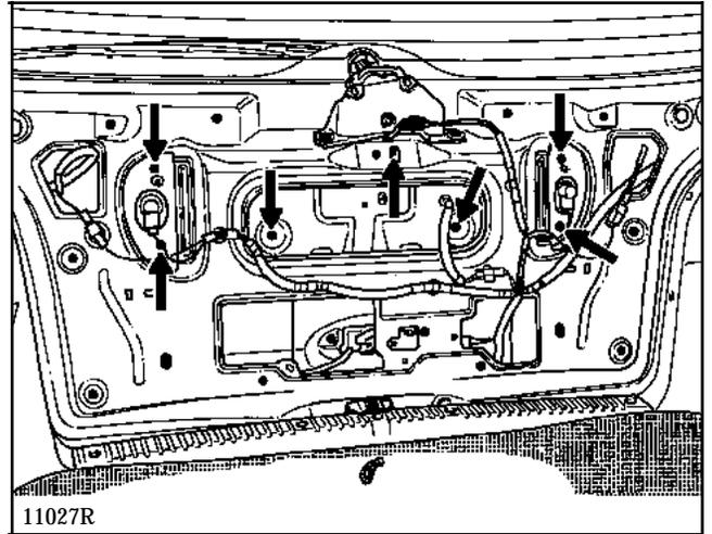
Unclip the strip at (F) and gently separate it from the vehicle to disconnect the connectors for the two number plate lights and release the wiring.
