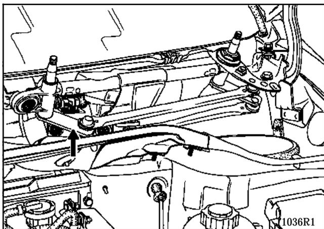
Disconnect and release the motor connector.
