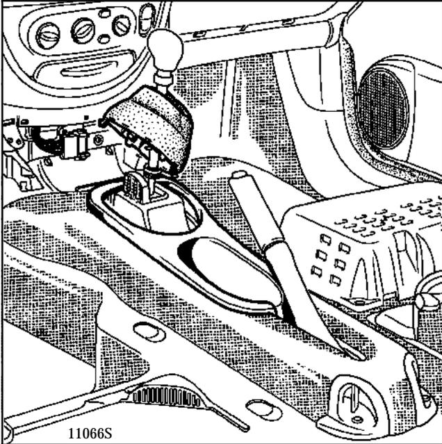
Remove the four mounting bolts from the console (two bolts at the front, two bolts at the rear).
