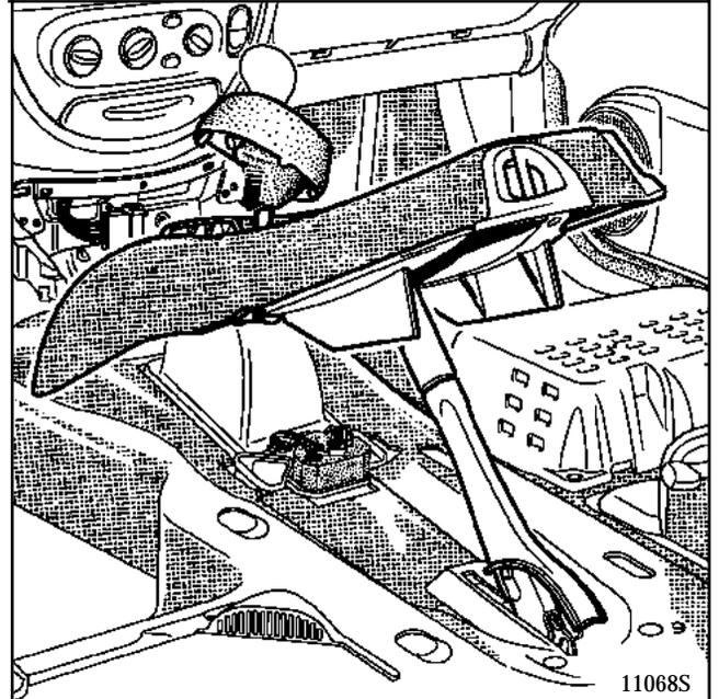
Disconnect the handbrake connector.
