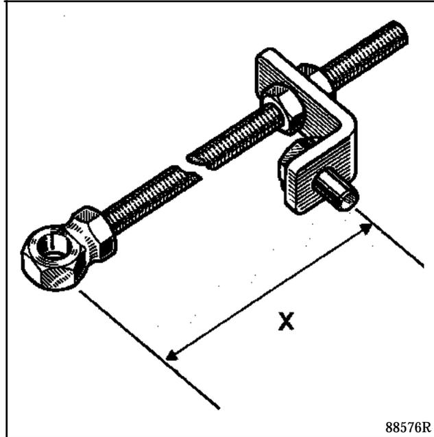
Fit the tool in place of the shock absorber.
