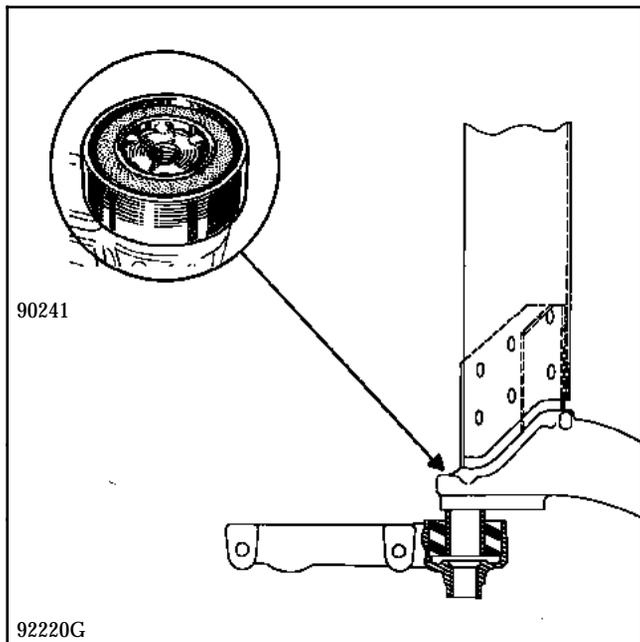
Remove the bush - bearing assembly on the press.
