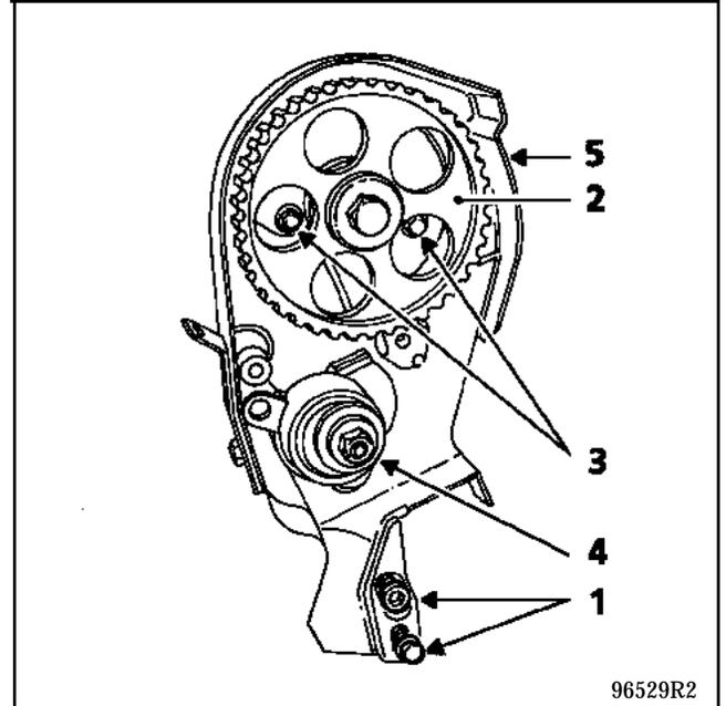
Remove the inner timing cover (5).
