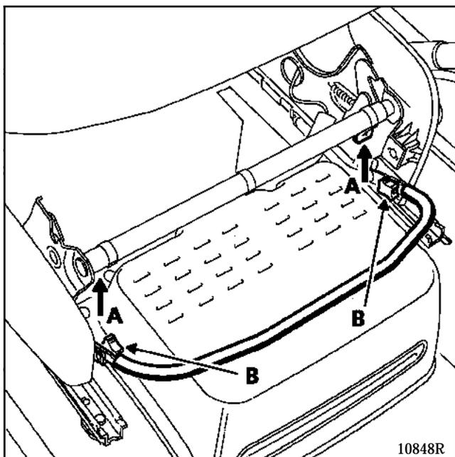
Slacken the two bolts (B) to lift the seat longitudinal position adjustment bar.
