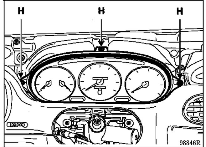
Remove the instrument panel, three bolts (H).
