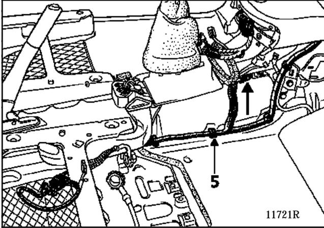
Release the wiring (5) on each side.
