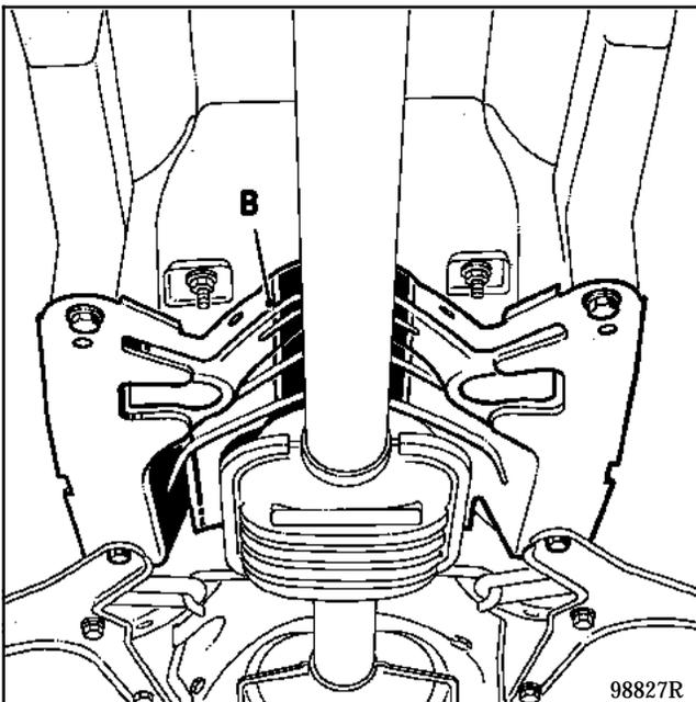
Note the handbrake adjustment dimension between the end of the rod and the caliper.
