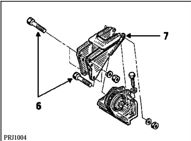
Remove the two mounting bolts from the power assisted steering on the sub-frame.
