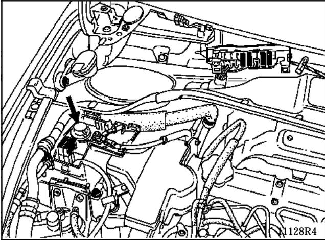
**This terminal only must be used** for jump-starting the vehicle (using the battery from another vehicle) and for recharging the battery. When recharging the battery, use an approved charger and an automatic charging programme with constant voltage to avoid over-consumption of electrolyte.
