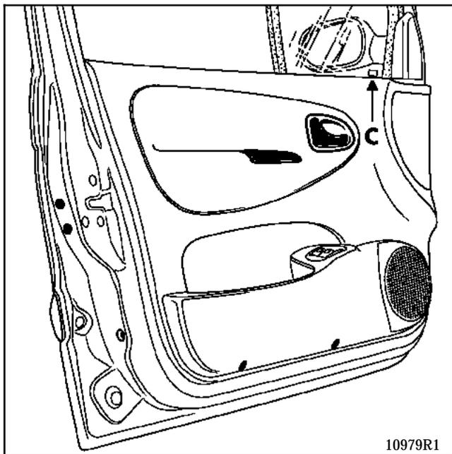
Unclip control (C) by pressing the tabs (D).
