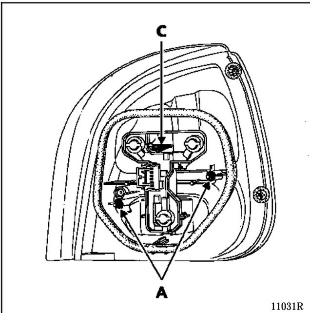
To reach the bulbs, unclip the bulb holder by pressing tab (C).
