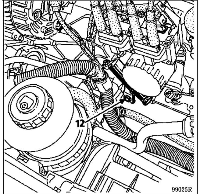
Fit the bracket of tool **Mot. 1159** under the water pump.
