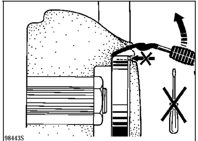
Separate the foam from the steering wheel in the centre, so that tool **Facom D115** may be correctly positioned.
