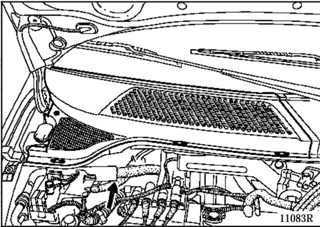
Remove the two retaining bolts for the pressure relief valve on the evaporator following the same method as above.
