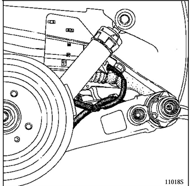
Disconnect the sensor connector located under the vehicle.
