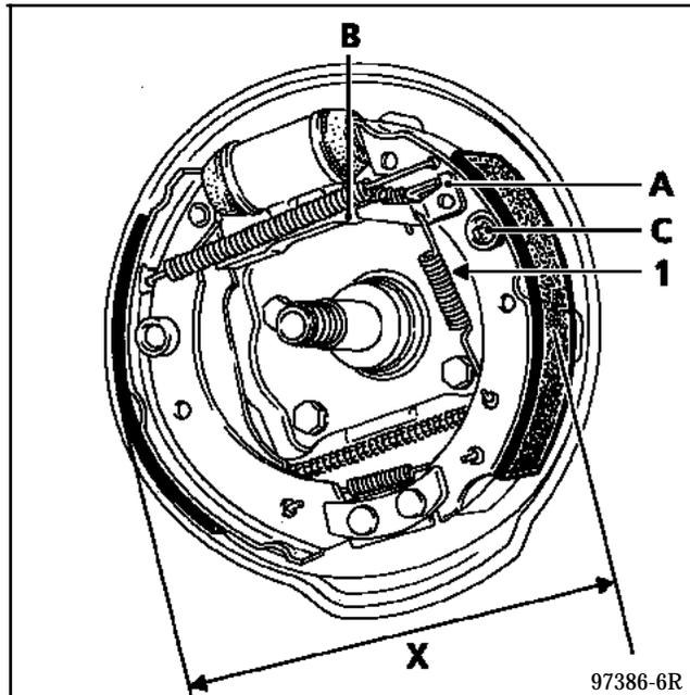
Check the ends of the lower and upper springs are correctly positioned on the shoes.
