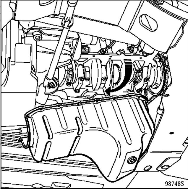
Clean the sump before applying a bead of RHODORSEAL 5661 of width 3 mm.
