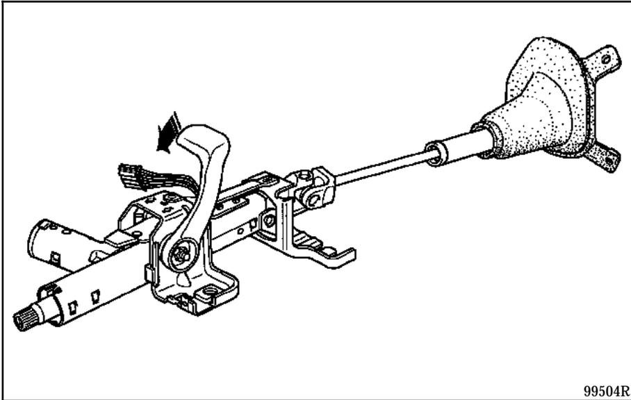
Remove the handle from the cams on the plastic washer (C) and turn it so that it is parallel to the steering column tube at the steering wheel end.
