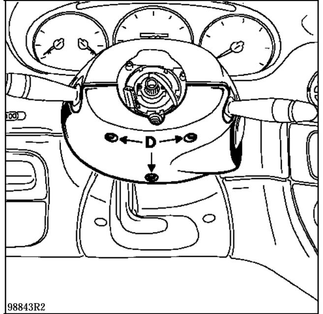
Remove the half cowling under the steering wheel by the three bolts (D).
