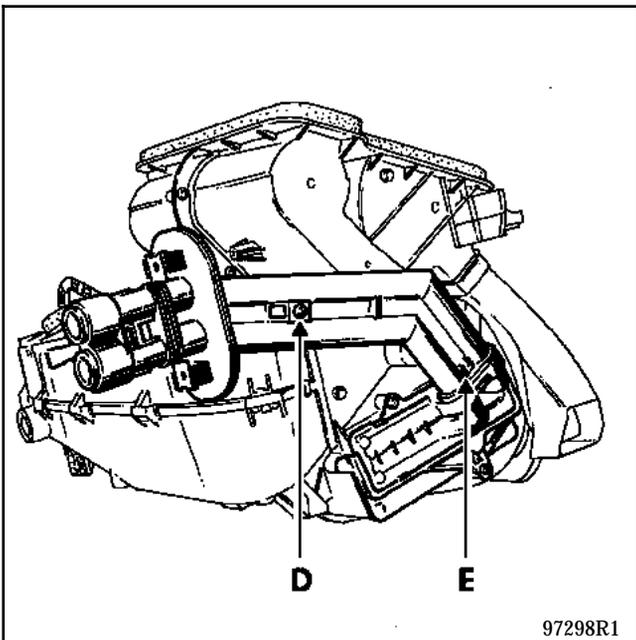
Separate the water downpipe from the heater matrix.
