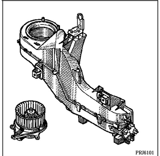
Release the fan assembly, then turn it anti-clockwise through 90° to remove it.
