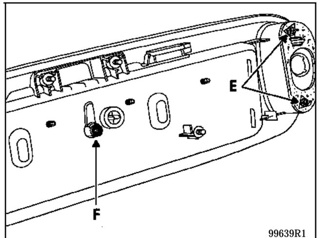
Remove the fog light(s) by slackening the two nuts (E).
