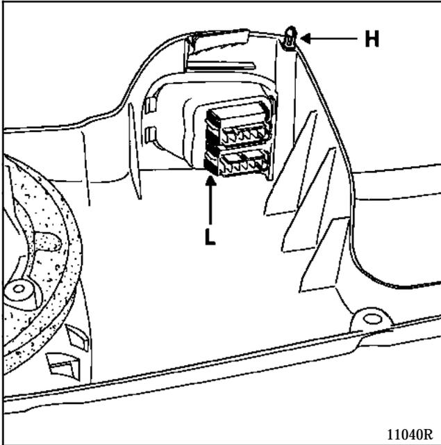
**NOTE :** a marking on each unit notes the connector colour to which it is connected. In addition, foolproofing on the tab clips ensures each unit is correctly refitted to the mounting plate.
