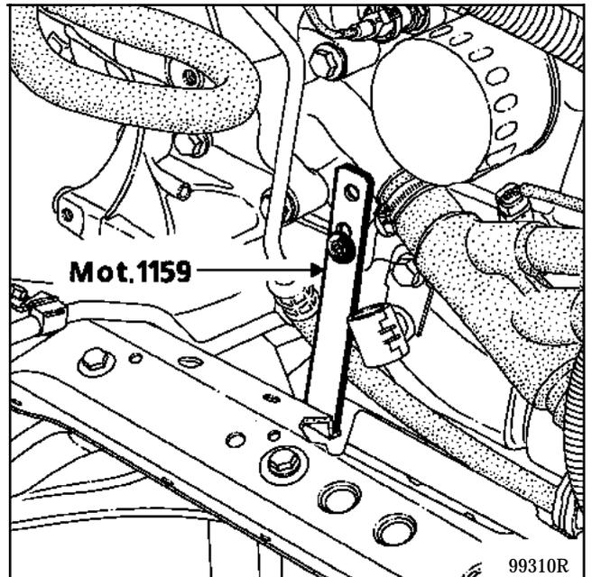
Diagram for drilling tool Mot. 1159
