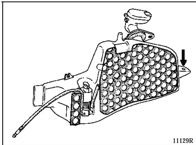
**ATTENTION :** When removing, disconnect the pump making sure that the two front and rear screen wash pipes are identifiable.
