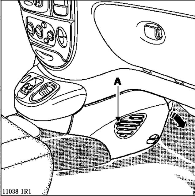
Remove the mounting bolt (A) for the side vent (on each side).
