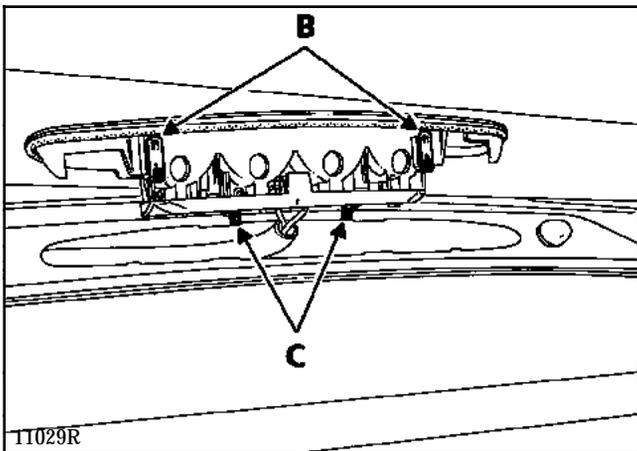
Lower the tailgate and release the light unit to the outside.
