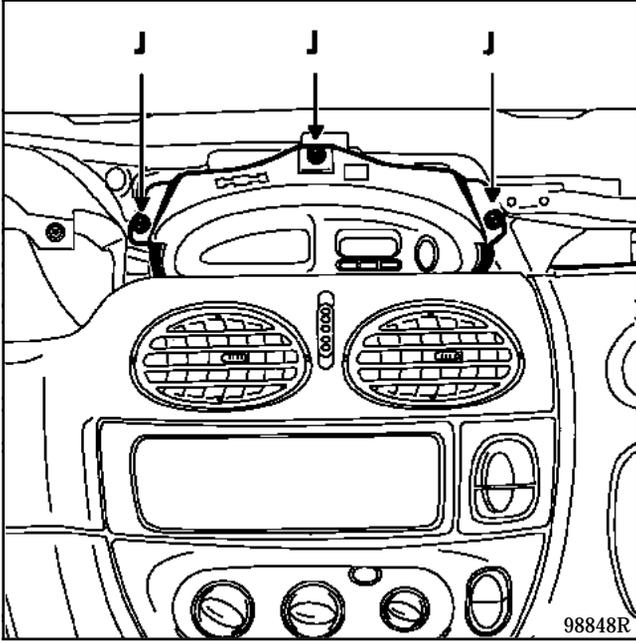
Remove the clock, three bolts (J).
