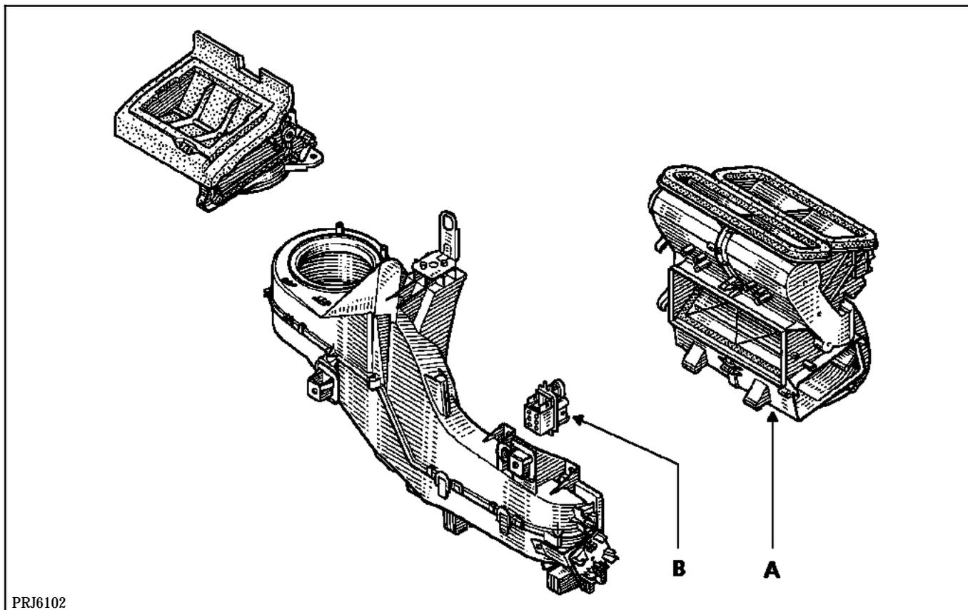
The distribution unit (A) may be reached after removing the dashboard.
