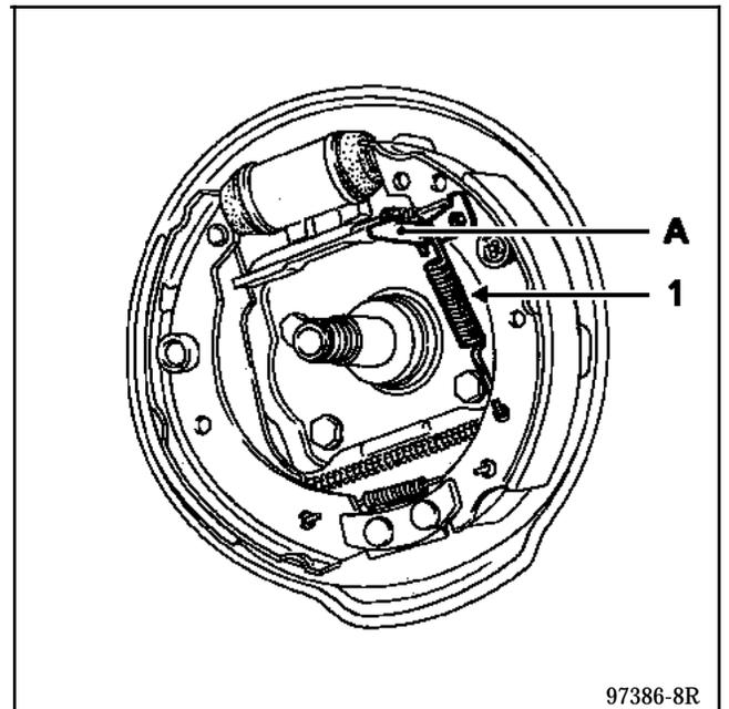
Fit a clamp on the wheel cylinder pistons.
