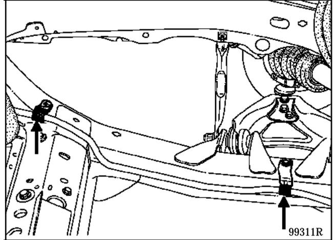
Lift the engine using the ring on the timing side until you obtain dimension (A) of 25 cm between the sub-frame and the edge of the cylinder block.
