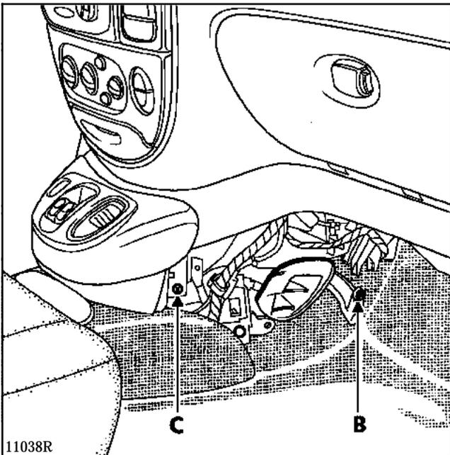
Remove the two mounting bolts (C).
