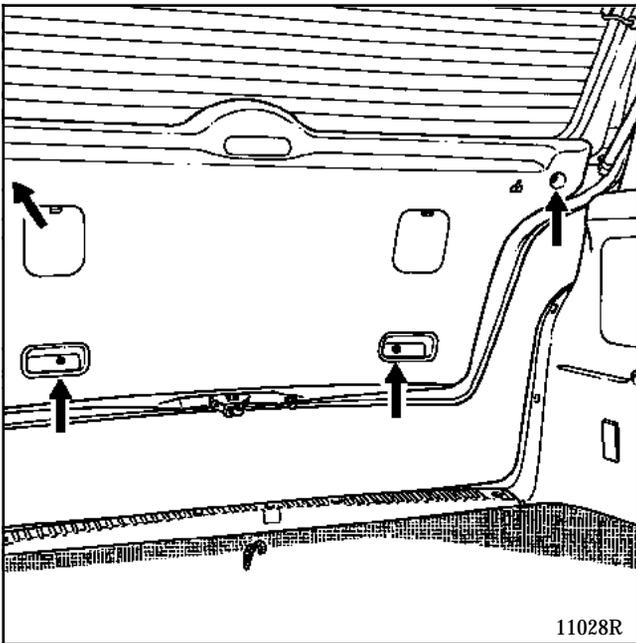
Unclip the trim, eleven clips secure it around the edge.
