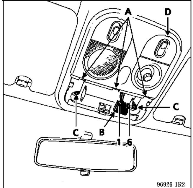
Remove the two mounting bolts (C) and release the roof console towards the front of the vehicle.
